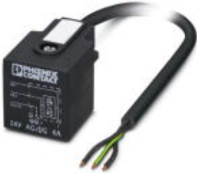
Sensor/Actuator cable, 3-position, PVC, Black RAL 9005, Free cable end, on A valve plug, with 1 LED, connected with Z diode, Cable length: 5 m
