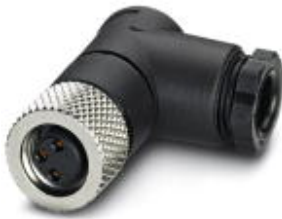
Sensor/actuator connector, female, angled, 3-pos., M8, solder connection, metal knurl, cable diameter max. 5 mm
