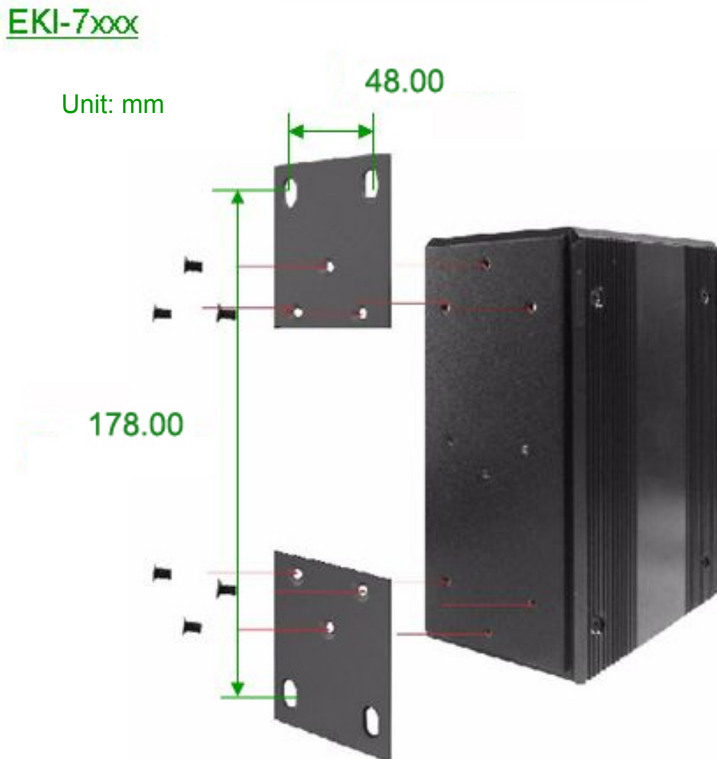
Figure 2.3-1 Combine the Metal Mounting Kit
