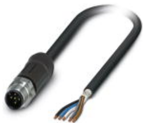
Sensor/Actuator cable, 5-position, PE-X/PE-X halogen-free, black-gray RAL 7021, shielded, Plug straight M12, A-coded, on free cable end, Cable length: 2 m, for outdoor applications, with high-grade steel knurl
