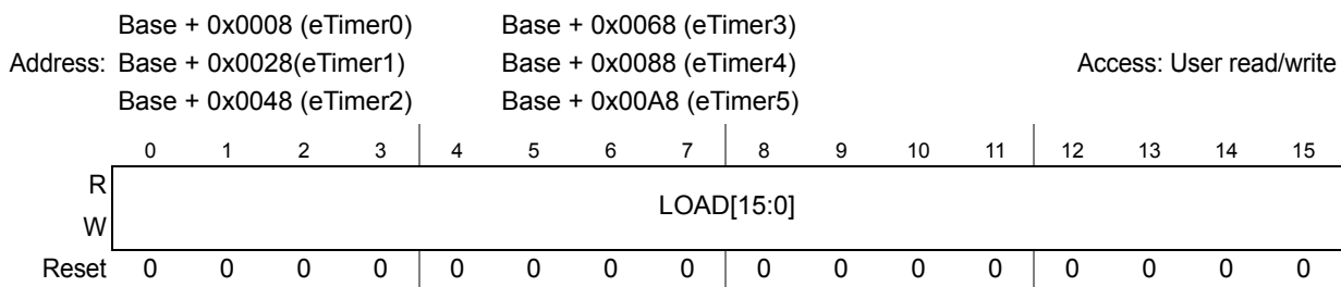
Figure 531. Load register (LOAD)
