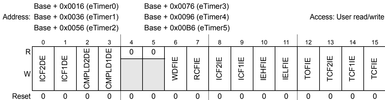
Figure 538. Interrupt and DMA enable register (INTDMA)
