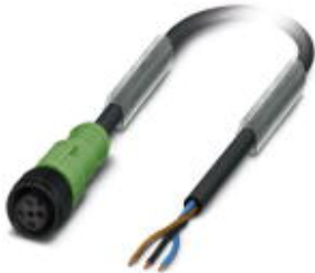
Sensor/Actuator cable, 3-position, PUR halogen-free, Black-gray RAL 7021, Free cable end, on Socket straight M12, A-coded, Cable length: 10 m, with plastic knurl
