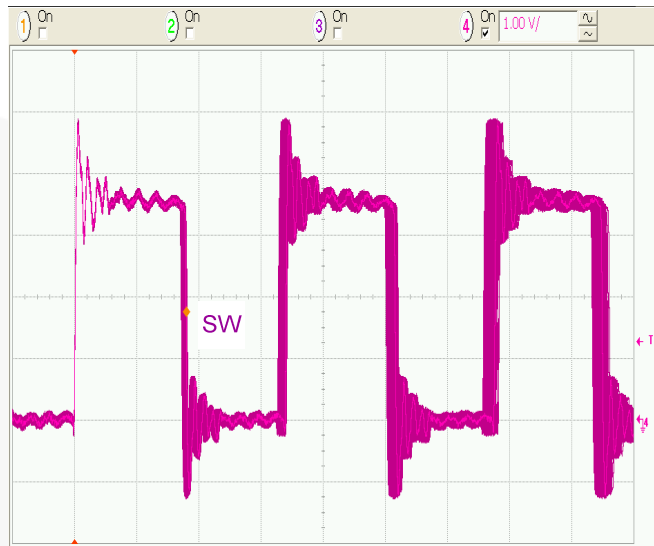
Figure 39. SW-Node Jitter (Infinite Persistence), I_{LOAD} = 200mA , 50ns/div .
