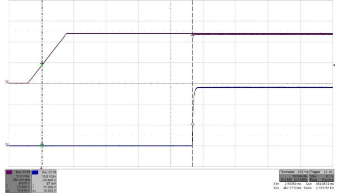
Fig. 29: Turn-on by Vin transient (ON/OFF high) at full rated load current (resistive) at Vin = 24V. Top trace (C2): Input voltage Vin (10 V/div.). Bottom trace (C4): Output voltage (10 V/div.). Time: 100 ms/div.
