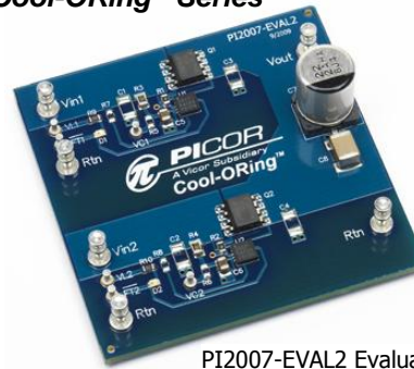
PI2007-EVAL2 Evaluation Board featuring the Cool-ORing PI2007 Active ORing controller.
