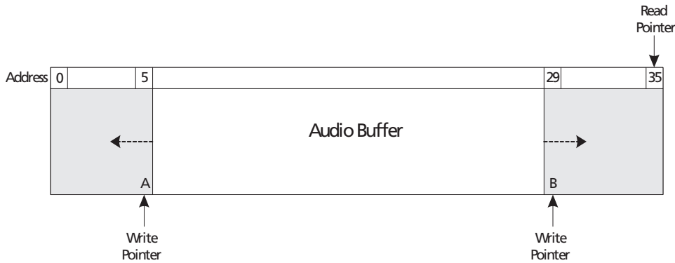
Figure 4-49: Audio Buffer Pointer Boundary Checking
