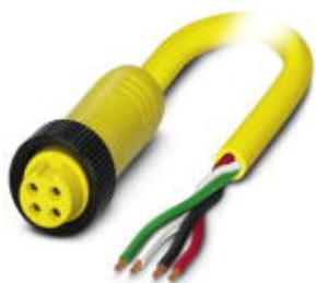
Power cable, 4-position, PVC, yellow, free cable end, A - standard, on Socket straight 7/8"-16UNF, cable length: 1 m
