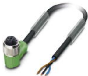
Sensor/actuator cable, 3-position, Variable cable type, free cable end, on Socket angled M12, A-coded, PIN 2+4 bridged, cable length: Free input (0.2 ... 40.0 m)
