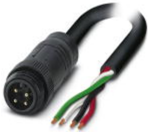
Power cable, 4-position, PVC, black, Plug straight 7/8"-16UNF, A - standard, on free cable end, A - standard, cable length: 10 m
