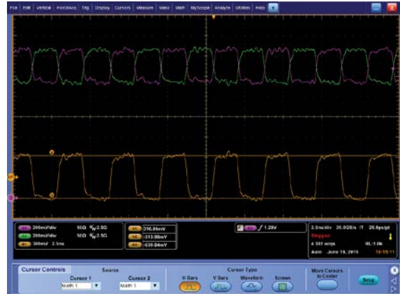
Figure 3. D_{OUT1-} and D_{OUT1+} with a 300 MHz Clock, Single-Ended and Differential
