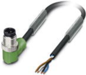
Sensor/actuator cable, 4-position, PUR halogen-free, black-gray RAL 7021, Plug angled M12, A-coded, on free cable end, cable length: 10 m
