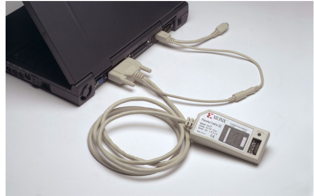
Figure 7: Laptop PC4 Cable Connection
