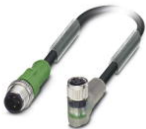
Sensor/actuator cable, 3-position, Variable cable type, Plug straight M12, A-coded, on Socket angled M8, with 2 LEDs, cable length: Free input (0.2 ... 40.0 m)
