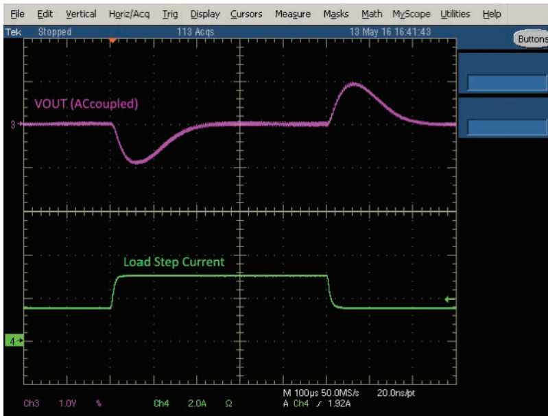
Figure 6. Load Transient Response (Conditions: V_{PORT} = 44V , Load Step: 1.5A to 3A to 1.5A)
