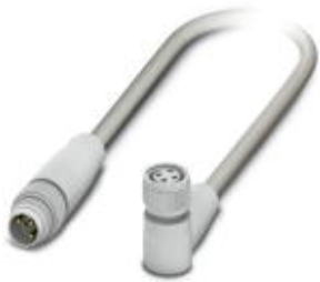
Sensor/Actuator cable, 3-position, PP-EPDM halogen-free, gray RAL 7035, Plug straight M8, on Socket angled M8, Cable length: 3 m, Hygienic design, with plastic knurl
