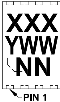
8-Lead UDFN (2x3x0.5 mm)
