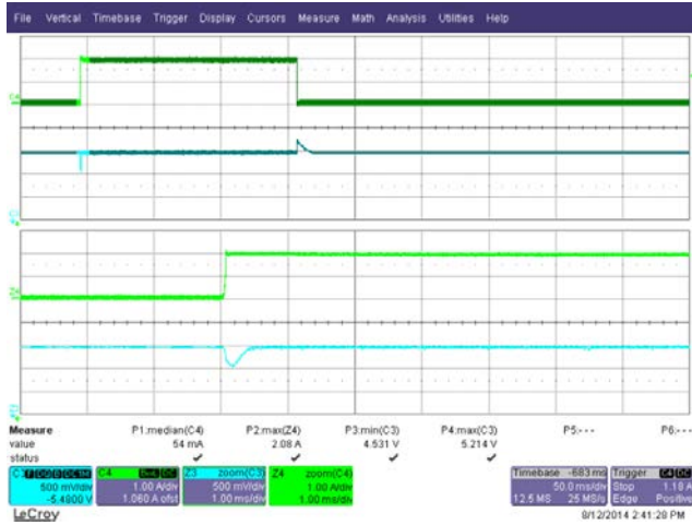
Figure 22 – Transient Response (4.5 V MIN ). 85 VAC, 0-2 A Load Step. Upper: I LOAD , 1 A / div. Lower: V OUT , 500 mV, 50 ms / div.
