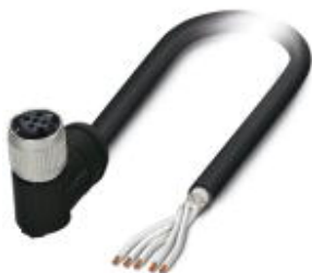
Sensor/Actuator cable, 5-position, PE-X halogen-free, black, shielded, free cable end, on Socket angled M12 SPEEDCON, A-coded, Cable length: 10 m, For railway applications
