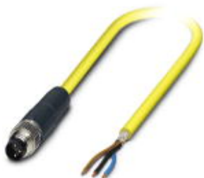
Sensor/Actuator cable, 3-position, PVC, yellow, shielded, Plug straight M8, on free cable end, Cable length: 2 m
