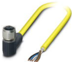
Sensor/Actuator cable, 5-position, PVC, yellow, shielded, free cable end, on Socket angled M12 SPEEDCON, A-coded, Cable length: 2 m
