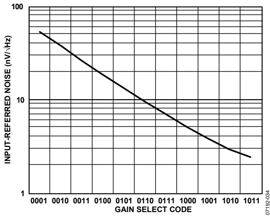
Figure 34. Input-Referred Noise vs. Gain Select Code for the VGA/Preamplifier See Figure 61
