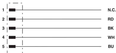
Contact assignment of the 7/8" plug
